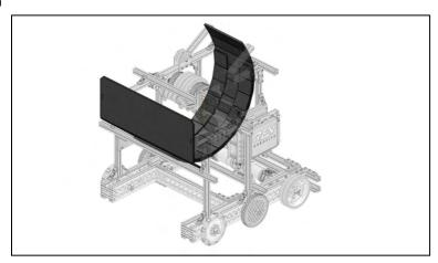
Insert the Corrugated Plastic Hopper and Hood as shown.
