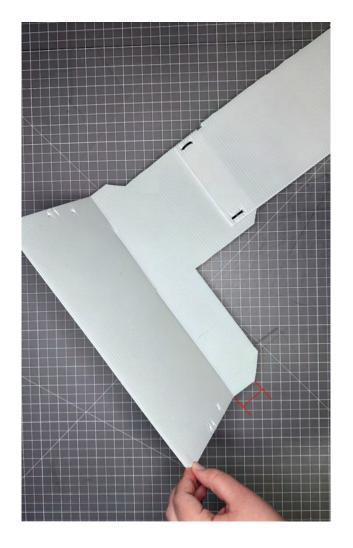
From the angle indicated in the photo, measure up 33mm and cut one side of Corrugated Plastic Sheet to allow for a smooth bend and form the Hopper.
