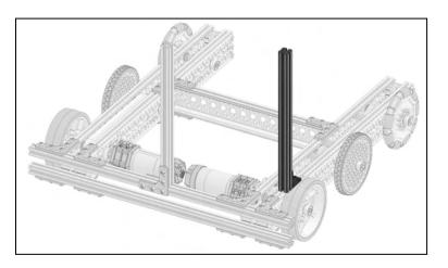
Slide the Inside Corner Bracket and Extrusion assembly on to the outer right rail of the Channel Drivetrain and secure.
