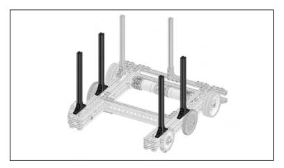
Slide on two Extrusion and Corner Bracket assemblies to each outer rail. Secure them in line with the centers of the Traction Wheels and Omni Wheels.
