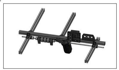
Slide Core Hex assembly on to the Agitator Assembly using the two Pillow Blocks to connect to the Extrusion.
