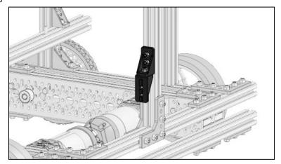
Slide on and secure the Lap Corner Bracket assembly from the previous step onto the Extrusion piece on the Drivetrain's back rail.
