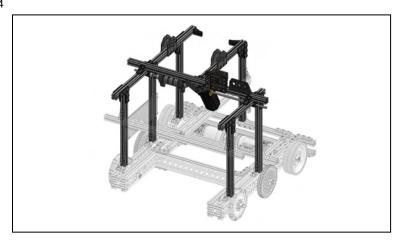
Slide Launcher Structure assembly on to the onto the Super Structure using the eight Plastic 90 Degree Brackets and two Inside Corner Brackets to connect to the Extrusion.
