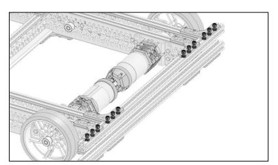
Loosen 12 screws on the back side of the Channel Drivetrain. Do not fully remove the nyloc nuts.
