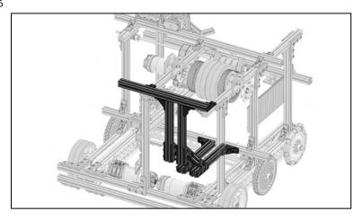
Slide the Hood Support assembly on to the onto the Super Structure using the two Inside Corner Brackets and two Lap Corner Bracket mounted in the previous step.
