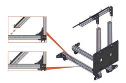
Add the 45 Degree Assembly to the Uprights. As you are sliding the 45 Degree Brackets down the Upright Extrusions add two M3 x 8mm Screws to **both** 15mm Extrusion - 150mm- 45° Ends. The screws should be on the same side of the Extrusions as the 45 Degree Brackets.
