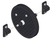
Sit two Bearing Pillow Blocks onto the Through Bore Bearings as shown.
