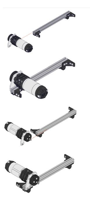
Add an UltraPlanetary Motor to the an External Cross Member by sliding the UltraPlanetary Flat Mounting Bracket through the Extrusion slot as shown. Adjust until the bracket is completely supported by the Extrusion. Tighten the Nylock Nuts until snug.
