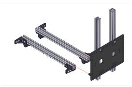
Add the Upright Assembly from above to the Internal Cross Members. Adjust until the Internal Cross Members are level with each other and the Upright Assembly is support on both Internal Cross Members. Tighten the Nylock Nuts until snug.
