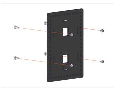
Pre-load four Hex Cap Screws and Nyloc Nuts per onto the Holder plate Battery Plate, as shown.
