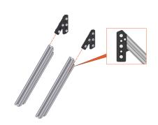
Add a Pre-Loaded 45 Degree Bracket to a 15mm Extrusion - 150mm- 45° Ends. The bracket should be set so that the vertex holes/screws are left exposed. Only 2 of the screws will be embedded into the Extrusion. Once placed tighten the Nylon Nuts on the bracket until snug.
