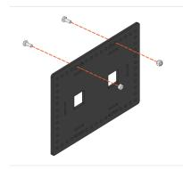
Pre-load two Hex Cap Screws and Nyloc Nuts per onto the Holder plate Battery Plate, as shown.
