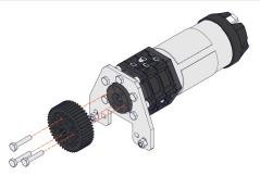
Attach a 45 Tooth Plastic Gear to the Output Cartridge using three M3 16mm Hex Head Screws. Tighten Screws until they are snug not tight.
