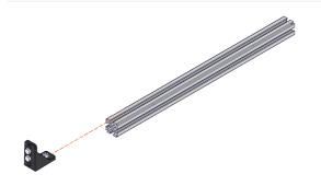
Slide a Pre-Loaded Inside Corner Bracket into the slot of a 15mm Extrusion - 225mm. Align the outer corner of the bracket with the end of the Extrusion. Tighten the Nylock Nuts until snug.
