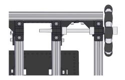
Slide the Omni Wheel Assembly through the Bearing Pillow Block on the nearby Internal Cross Member.
