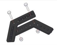
Attach two 120 Degree Brackets to each other using M3  $\,\mathrm{x}$  16mm Screws and Nylock Nuts as show. Tight the Nylock Nuts until snug.
