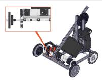
Slide a Touch Sensor, pre-loaded with M3 x 8mm Screws and Nylock Nuts, onto the Extrusion where the wheel was pulled out in the previous step. Adjust the Touch Sensor so that it is interacting with the Limit Switch Bumper on the arm.
