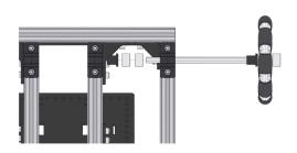
Slide a Omni Wheel Assembly through a an External Cross Member -Bearing Pillow Block, as shown. Add two Shaft Collars on the shaft and a Through Bore Bearing - Long. Both bearings should be facing toward the center of the chassis.
