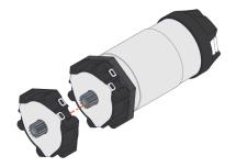
Seat the UltraPlanetary 4:1 Cartridge onto the UltraPlanetary 5:1 Cartridge.
