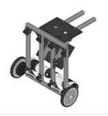
Repeat the previous steps to add the second Traction Wheel Assembly to the Robot Frame.
