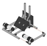
Add the Left Motor and Cross Member Assembly to the Internal Robot Frame Assembly. The outer edge of the Motor and Cross Member Assembly should be flush with the ends of the of the Internal Robot Frame Extrusions. Once adjusted tighten the Nylock Nuts on the Inside Corner Brackets until snug.
