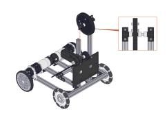
Slide the Bearing Pillow Blocks onto the Uprights. The upper edge of the Pillow Blocks should be flush with the top of the Extrusions. Tighten the Nylock Nuts on the Bearing Pillow Blocks.
