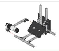
Add the Right Motor and Cross Member Assembly to the Internal Robot Frame Assembly. The outer edge of the Motor and Cross Member Assembly should be flush with the ends of the of the Internal Robot Frame Extrusions. Once adjusted tighten the Nylock Nuts on the Inside Corner Brackets until snug.
