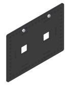
Once the screws have been pre-loaded onto the Battery Holder Plate, set the Battery Holder Plate aside.
