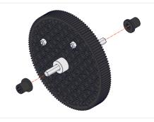
$\operatorname{\mathsf{Add}}\nolimits$  two Through Bore Bearing - Long to the shaft as shown
