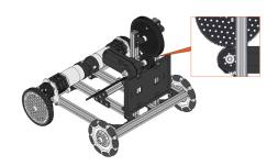
Adjust the Core Hex Motor Assembly so that the 45 Tooth Gear is meshed with the 125 Tooth Gear as shown.
