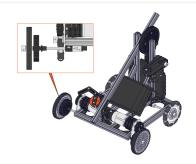
Loosen the Shaft Collars on one of the Traction Wheel Assemblies and pull the wheel partially out of the Bearing Pillow Blocks as shown.
