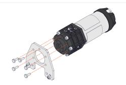
Attach the Pre-Loaded UltraPlanetary Flat Mounting Bracket to the Output Cartridge using five M3 x 8mm Hex Head Screws. Tighten Screws until they are snug not tight.
