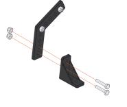
Attach an Inside Corner Bracket to the 120 Degree Bracket using two M3 x 16mm Screws and Nylon Nuts as shown. Tighten the Nylon Nuts until snug.
