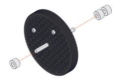
Add three Shaft Collars onto the shaft as shown. Leave the shaft collars loose for now so adjustments can be made later.
