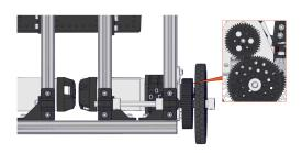
Slide the Traction Wheel Assembly through the Bearing Pillow Block on the nearby Internal Cross Member.
