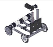
Slide the Core Hex Motor Assembly down the Upright Extrusion as shown. The Bent Core Hex Motor Bracket will be on the same side of the Upright as the Battery Holder plate.
