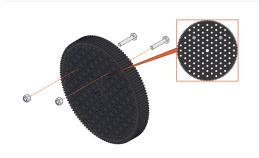
Attach to M3 x 16mm Screws to the 125 Tooth Plastic gear as shown in the image above.
