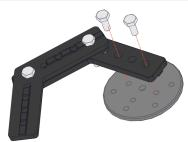
Attach the 120 Degree Bracket Assembly to the Aluminum Servo Horn using two M3 x 8mm Screws as shown. Tighten the screws until snug.
