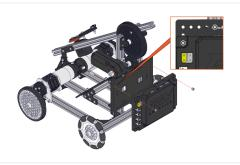
Attach the Control Hub to the Battery Holder Plate on the Uprights using two M3  $\times$  16mm Screws and Nyloc Nuts. The Control Hub should be mounted to the plate using the third hole from the top of the plate as shown. Tighten the Nylock Nuts until snug.
