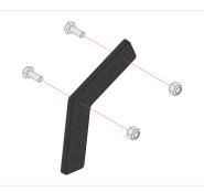
Attach two M3 x 8mm Screws to a 120 Degree Bracket as shown.
