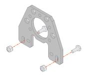
Take a bracket and finger start one Hex Cap Screw and Nyloc Nut per hole.
