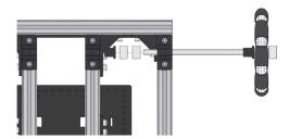
Slide a Omni Wheel Assembly through a an External Cross Member -Bearing Pillow Block, as shown. Add two Shaft Collars on the shaft and a Through Bore Bearing - Long. Both bearings should be facing toward the center of the chassis.
