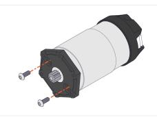
Attach the UltraPlanetary Mounting Plate to the HD Hex Motor using two 8mm Button Head Screws.
