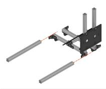
Add two 15mm Extrusion - 225mm to the Inside Corner Brackets of the Internal Cross Members, as shown. The rest of the Internal Frame (i.e. the Internal Cross Member, 45 Degree, and Upright Assemblies) should be centered on each Extrusion.
