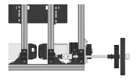
Slide a Traction Wheel Assembly through a an External Cross Member -Bearing Pillow Block, as shown. Add two Shaft Collars on the shaft and a Through Bore Bearing - Long. Both bearings should be facing toward the center of the chassis.
