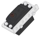
Attach the Servo to the Pre-Loaded Bent Servo Bracket using M3 x 8mm Screws and Nyloc Nuts. Tighten the Nylock Nuts until snug.
