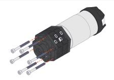
Insert six of the 30mm Cap Head Screws into the holes in the outer ring off the Output Cartridge.
