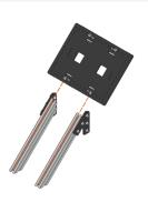
Add the two Pre-Loaded 45 Degree Bracket and 15mm Extrusion - 150mm- 45° Ends assemblies to the Battery Holder Plate from the start of this assembly. Adjust the Plate so that both Extrusion pieces are in line with each other. Tighten the Nylock Nuts until snug.
