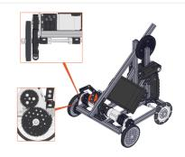
Slide the Traction Wheel Assembly back into its proper place. Before tightening the Shaft Collars make sure that the gear on the wheel assembly is meshed with the gear on the UltraPlanetary Motor.
