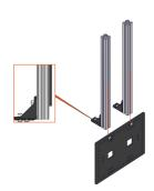
Add the two Pre-loaded Inside Corner Bracket and 15mm Extrusion - 225mm assemblies to the Battery Holder Plate from the start of this assembly. Adjust the Plate so that both Extrusion pieces are in line with each other. Tighten the Nylock Nuts until snug.
