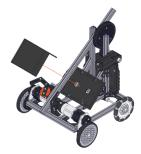
Use Hook and Loop Fastener to attach at 12V Slim Battery to the Battery Holder Plate on the 45 Degree Assembly.
