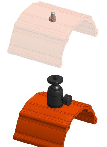
Insert the Camera Mount bolt through the Wheel Cover aligning the bolt head with the grooves in the Wheel Cover. Then screw the Camera Mount onto the bolt.
