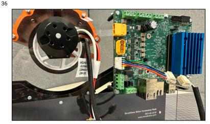
Connect the NEO 550's Sensor cable to the K24 SOM Development Board.
