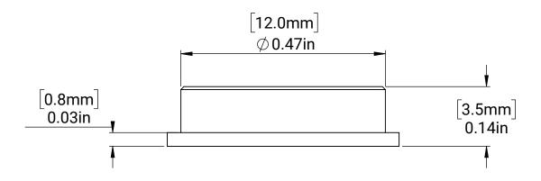
MM SHEET TOLERANCES: X ± 0.50 MM X.X ± 0.10 MM X.XX ± 0.05 MM ANGLES ± 2° INCH SHEET TOLERANCES: X ± 0.1 IN X.X ± 0.02 IN X.XX ± 0.004 IN X.XXX ± 0.002 IN ANGLES ± 2° MATERIAL:
