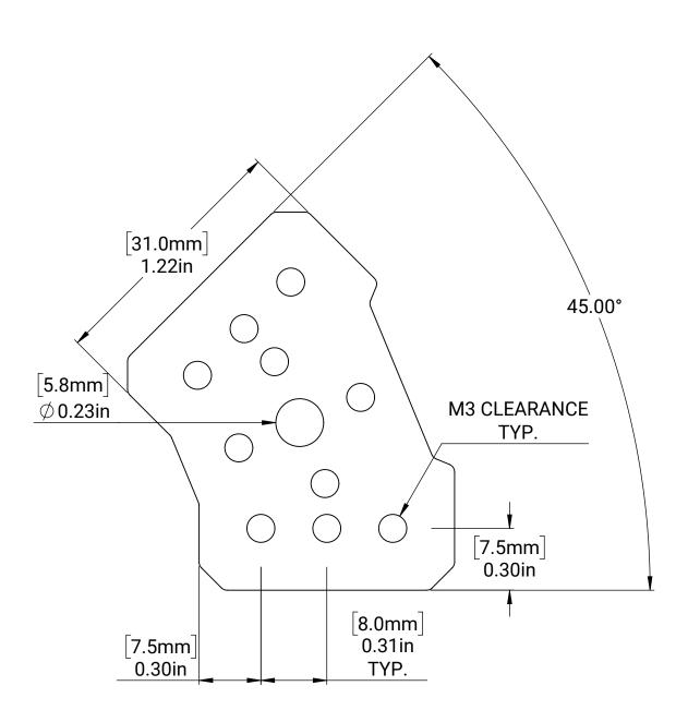
MM SHEET TOLERANCES: X ± 0.50 MM X.X ± 0.10 MM X.XX ± 0.05 MM ANGLES ± 2° INCH SHEET TOLERANCES: X ± 0.1 IN X.X ± 0.02 IN X.XX ± 0.004 IN X.XXX ± 0.002 IN ANGLES ± 2° MATERIAL:
