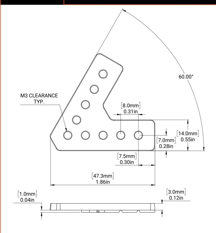
MM SHEET TOLERANCES: X ± 0.50 MM X.X ± 0.10 MM X.XX ± 0.05 MM ANGLES ± 2° INCH SHEET TOLERANCES: X ± 0.1 IN X.X ± 0.02 IN X.XX ± 0.004 IN X.XXX ± 0.002 IN ANGLES ± 2° MATERIAL: **NYLON**
