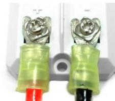
The Servo Power Module has two screw terminals for 12V power input. It is recommended to use ring or fork terminals designed for #6 or M3 screw terminals.
