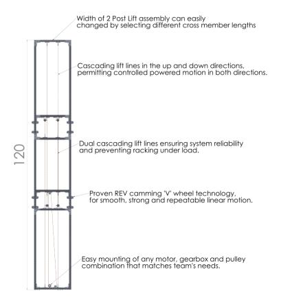
Extremely compact cross section enabling teams to dedicate valuable robot real estate to drivetrain and manipulator.
