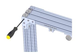
Tighten\* the screws starting with the 1st Stage screws. Be sure to confirm that the Cross Members are in the correct locations and square with the vertical 48" Long 1" REV Extrusions.
