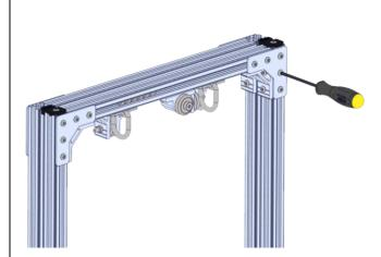
Tighten\* the screws starting with the 1st Stage screws.
