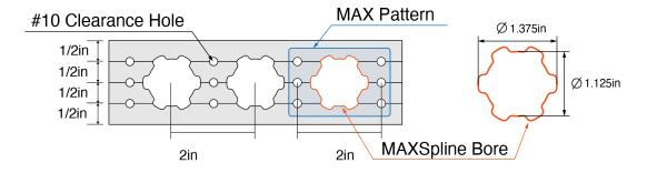
MAXTube's Grid Pattern is featured on two sizes of MAXTube: 1x1 and 2x1. A grid of #10 clearance holes are spaced along each side of the MAXTube on a 1/2in pitch.
