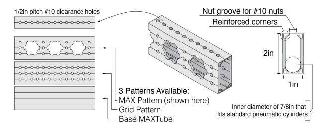
MAXTube with MAX Pattern features a combination of #10 clearance holes and a MAXSpline bore patterned every 2in. The #10 clearance holes are arranged on a common 1/2in pitch grid. MAX Pattern frees teams from cutting and drilling, with easy installation of bearings for different live axle applications, as well as correct center-to-center distances for simple 1:1 power transmission with #25 chain or RT25 belts.
