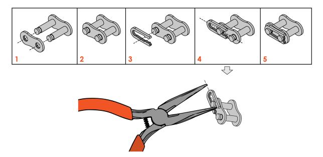
Instead of using a master link, REV's #25 Chain Tool can be used to push out a pin and then push the pin back in once the link has been formed for a stronger, but more difficult, joining method. For instructions on how to break and reassemble the chain using this method, see the *Chain Tool User's Manual* and 'How-To' video found on its product page on our website.
