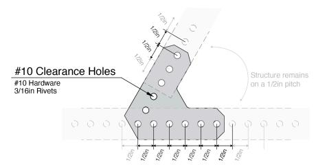
ION 1 in Brackets are hole-aligned to maintain the pitch grid between your MAXTubes. When building a robot with hole-aligned brackets, you will likely notice an open space between the structure ends, where they do not touch at the corner. This is expected and will not affect the strength of your joint.
