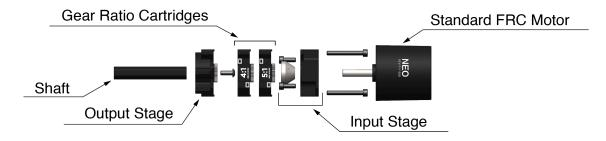
A wide range of gear ratios are possible with the three available cartridges. When combining up to three cartridges, just multiply each cartridge gear ratio to find the overall gear ratio. For example, a combination of the 4:1 and 5:1 cartridges make a 20:1 overall gear ratio. The table below shows the common use cases for all possible ratios that can be created with the MAXPlanetary Gearbox.
