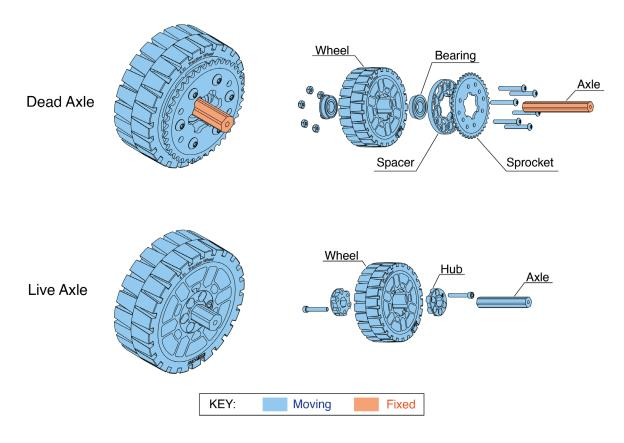
In the REV ION Build System, MAXHubs provide a way to transfer torque to a MAXSpline Bore from shafts of various shapes and sizes. MAXHub variants allow for other bores or mount holes to populate within an existing MAXSpline.
