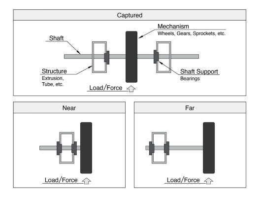
Additionally, the further apart the two support points are from each other, the better it can resist effects of a normal force. As the supports move closer together, they begin to act more like a single support.
