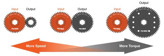
To ensure that you have a proper amount of gear teeth mesh, it is important to calculate the center-to-center distance in between your gears. You can do this by first calculating the pitch diameter (PD) of each gear using some combination of module (M), number of teeth (N), or outside diameter (OD).
