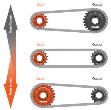
Chain Loops can be used with ION Sprockets and structure featuring the MAX Pattern. Any 1:1 ratio will have the correct center-to-center distance for a properly tensioned chain, without the need for tensioning bushings. To calculate how many links you will need, multiply the center-to-center distance by eight, and add the number of teeth on one sprocket.
