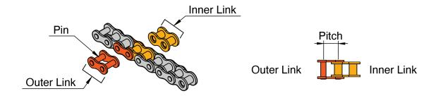
Creating a loop of chain requires breaking off the correct number of links by removing a specific chain pin and joining the ends together. Chain can be broken using many methods, including a Chain Tool or various steel cutting blades, like a dremel. Once you have counted the number of links necessary for your application, the chain can be joined using a master link or by replacing a pin. The diagram below shows how a master link is assembled to replace an outer link.
