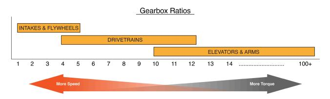
While this table is a good starting point, please take a look at the *MAXPlanetary Gearbox User's Manual* on our website before configuring the gearbox. The guide contains detailed information about the system features and limitations that are very useful when designing a robot. The online documentation also has information about how the type of motor used will affect what ratios are effective for different mechanisms.
