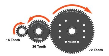
Transforming the torque and speed of motion can be accomplished by changing the size of the gears.
