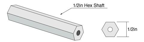
Sometimes when building with 1/2in hex shaft, it can be difficult to line up the shape within hex bore elements because the corners must be perfectly aligned. 1/2in Rounded Hex Shaft is a popular variation of 1/2in hex shaft. With the corners rounded to form a 13.75mm circle, 1/2in Rounded Hex Shaft pilots smoothly inside 1/2in hex bore components as well as standard 1.125in flanged bearings for an easy assembly experience.
