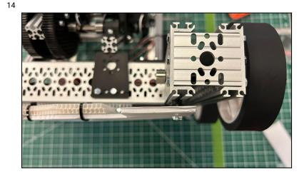
Proceed to install the Intake Stabilizer on the C Channel cavity, you should line the plastic up with the front ends of the robot so that they are flush.
