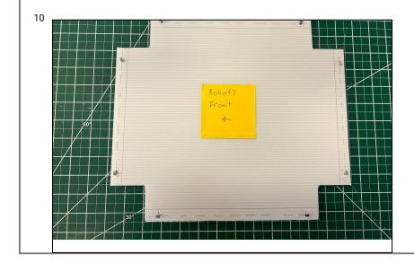
Once you have your plastic sheet cut to the appropriate dimensions and have punctured all eight holes we can move to installing the belly pan to the bottom of the starter bot.
