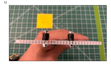
Insert the three spacers on the screw, then install the screw through the hole. Similar to the belly pan, thread the Nyloc nut on the screw but not all the way.
