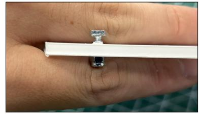
Be sure to load the Nyloc Nut onto the T-Slot Screw just enough so that you can push the screw up, you should have the head sticking out a little. This will allow the screw to catch the extrusion and fasten correctly and prevent the hardware from free spinning in the plastic.
