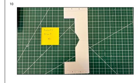
Find the center of the outlines you have made and mark two dots at 35mm apart.
