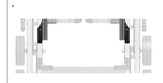
Fasten the preloaded Gearbox Motion Bracket to the Channel Drivetrain.
