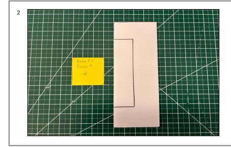
Cut the excess plastic along the vertical left 278mm line.
