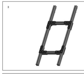
• 2 - 15mm Extrusion - 120mm - 90° Ends
