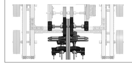
Attach the Gripper Assembly to the Arm Assembly by removing both the Bearing Pillow Blocks from the Arm Assembly and sliding them onto the Gripper Assembly shaft. Then slide the Bearing Pillow Blocks back into place connecting the gears on the Gripper Assembly to the Arm Assembly.
