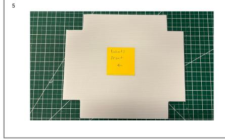
With the shape of your belly pan now completed we'll move on to tracing outlines for the M3 Hardware.
