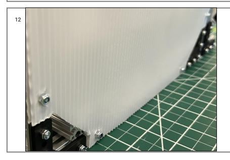
Line up the belly pan so that the T-Slot Screws go into the 15mm Extrusion cavity. Begin to fasten all eight preloaded M3 hardware points to the bottom of the robot.
