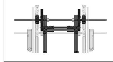
Attach the Arm Assembly to the Tower Assembly by loosening the Metal Bent Core Hex Motor Brackets, removing both the Bearing Pillow Blocks from the Tower Assembly and sliding them onto the Arm Assembly shaft. Then Slide the Bearing Pillow Blocks back into place connecting the gears on the Arm Assembly to the Tower Assembly. Then reattach the Metal Bent Core Hex Motor Brackets.
