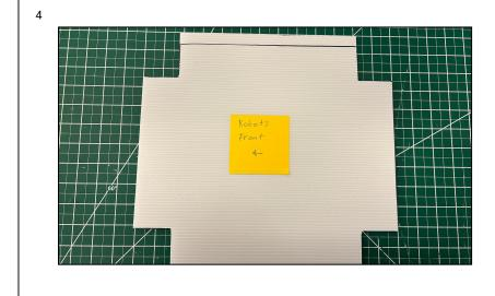
With all four corners removed, cut the excess plastic from the top.
