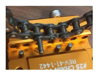
Put the Inner Link bushing into the Outer Link. Align the Pin in the Compression Screw hole.
