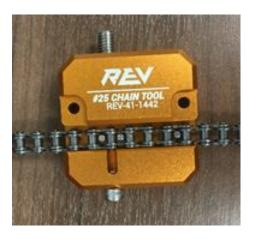
Insert #25 chain into the chain channel and align the desired link between the two vertical pins in the channel.
