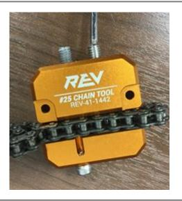
Turn the Compression Screw until the Pin is fully seated back into the chain channel.
