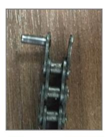
Screw the Pin Screw down until the pin almost touches the Cup Point Set Screw. The user should stop pushing the pin out before it leaves the back plate the outer link. Considerable pressure will be felt before the pin comes all the way out. Removing the chain from the tool to check if the pin is fully unseated from the bushing is recommended.
