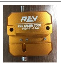
Unscrew the Pin Screw and Compression Screw such that they are flush with the chain channel.
