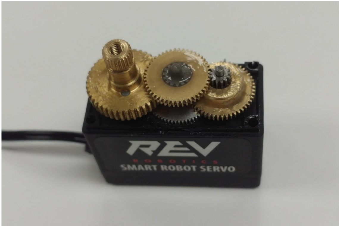
Figure 11: Place the final gear on the middle shaft. It should first mesh with the output shaft on its lower set of teeth, and then its upper teeth will mesh with the gear on the right shaft.
