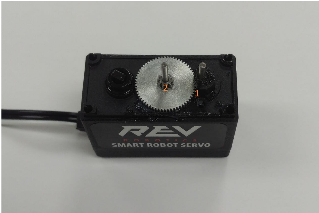
Figure 7: Place the new silver gear onto the servo unit. (1) Make contact with the servo motor's output shaft gear first, then (2) slide the axle into the plastic axle hole.
