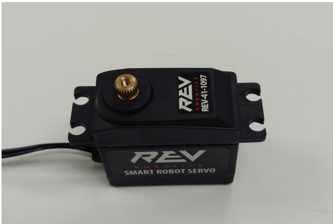
Figure 12: Finally, reattach the top plastic cover, making sure to place it directly down on top of the gears so that they don't become misaligned. Reattach the 4 screws and the servo is ready to operate.
