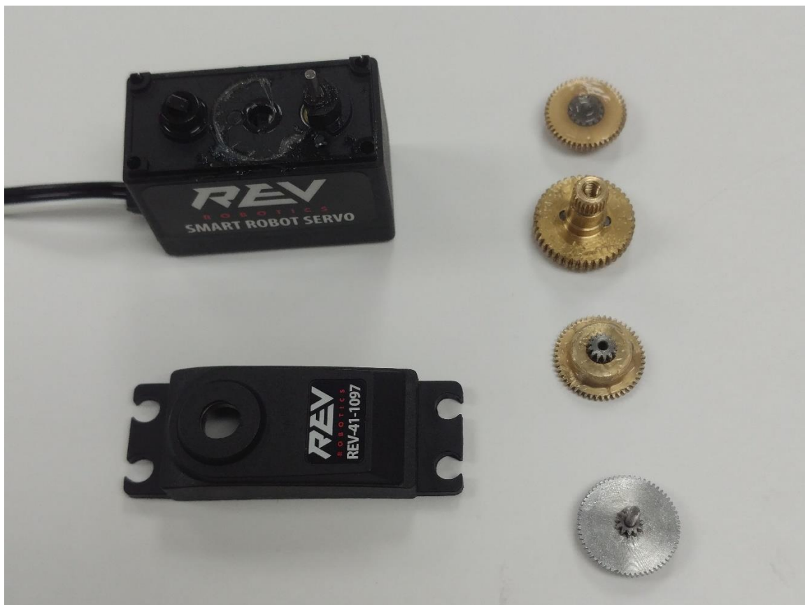
Figure 3: Take off top plastic cover of servo.
