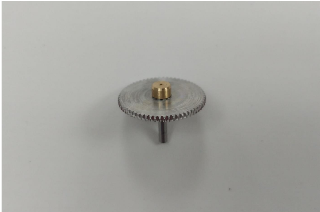
Figure 6: Attach the new silver gear to the axle pin.
