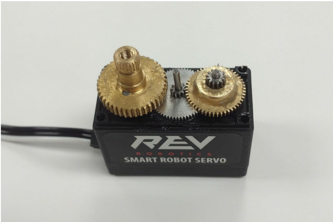
Figure 10: Once the output shaft is in place correctly, it should be seated securely but not touching any other gears.
