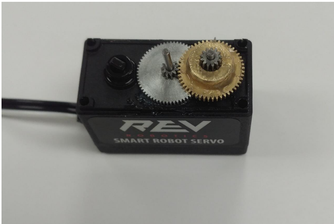
Figure 8: Place the second gear in place. Make sure the lower level of teeth on this gear mesh with the upper level of teeth on the silver gear.
