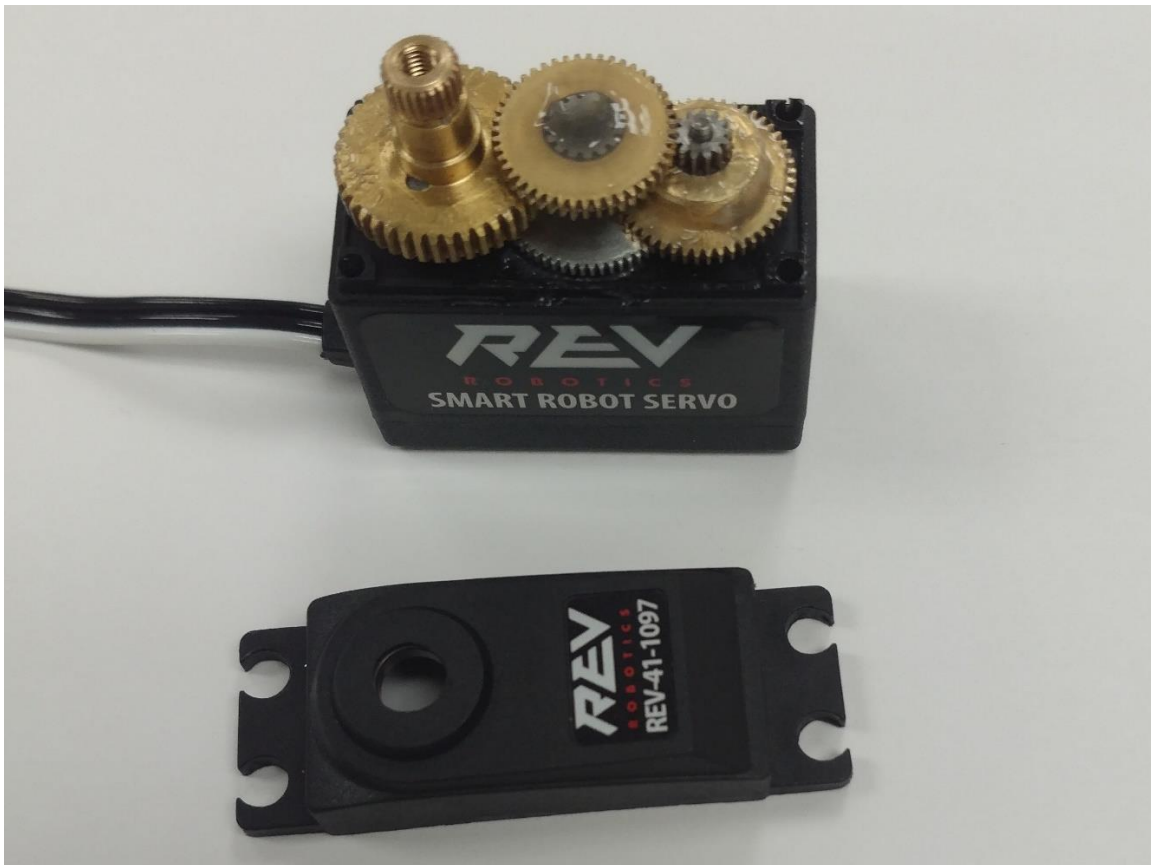
Figure 3: Take off top plastic cover of servo.
