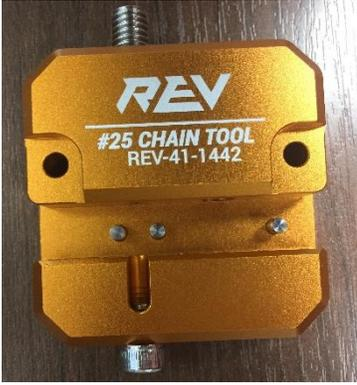
A close-up photograph of the REV #25 Chain Tool (REV-41-1442). The tool is orange and has a central channel. The top and bottom screws are loosened and are not flush with the channel.                                                    | <p style="text-align: center;"><b>Step 1</b></p> <p>Unscrew the pin screw and compression screw such that they are flush with the chain channel.</p>                                   |
