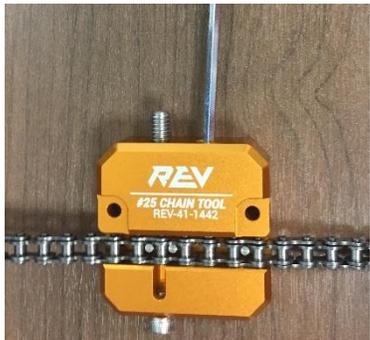
A close-up photograph of the REV #25 Chain Tool (REV-41-1442) with the #25 chain (REV-41-1365) inserted. The chain is now secured in place by the compression screw, which is tightened until the chain cannot shift within the channel. | <p style="text-align: center;"><b>Step 3</b></p> <p>Next secure the chain in place with the compression screw. Tighten until the chain cannot shift within the channel.</p>            |
