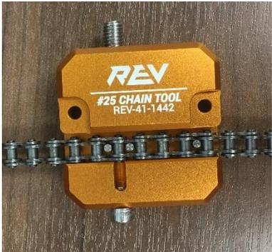
A close-up photograph of the REV #25 Chain Tool (REV-41-1442) with a #25 chain (REV-41-1365) inserted into the channel. The chain is positioned between two vertical pins in the channel.                                                 | <p style="text-align: center;"><b>Step 2</b></p> <p>Insert #25 chain (REV-41-1365) into the chain channel and align the desired link between the two vertical pins in the channel.</p> |
