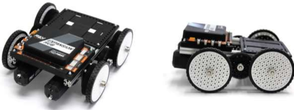
Figure 4: The miniBot is a Simple 2-Motor Robot
