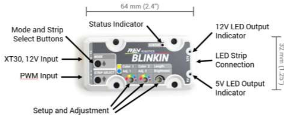
Figure 1: Blinkin Connections and Indicators
